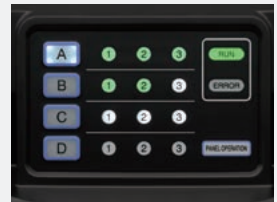
Signaled by white light for correctly loaded cassettes, blinked white light for incorrectly loaded cassettes, green light for the completion of scanning.
